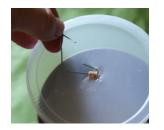
8. Roll the can under your hand to see if the battery touches the side of the can. If it does, tighten the rubber bands.
